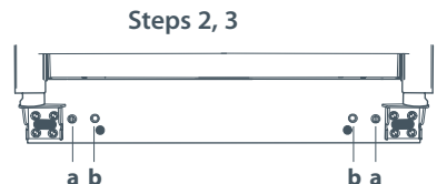
Fig.5 Levelling the refrigerator
